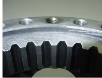
CHAMFERED FACE ON END OF SPLINES
